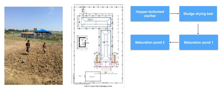
Figure 14. Sludge treatment facilities in Kyein Ni Phin, Pauktaw; site plan; and sludge treatment process (DRC, 2018)
