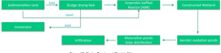
Figure 12. Sludge Treatment Plant in Sittwe (Solidarites International, 2018)
