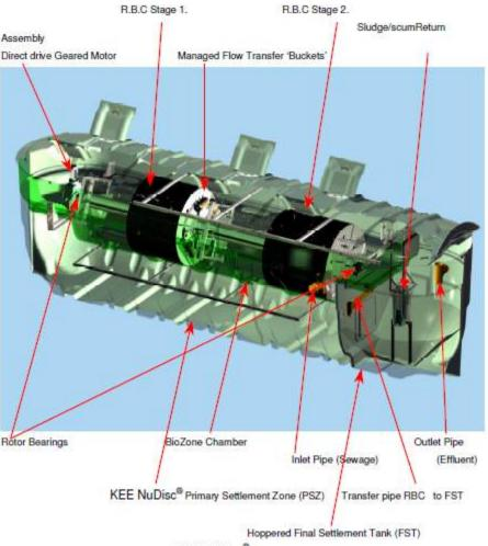
FIG 1: Cut through of KEE1600 KEE NuDisc<sup>®</sup> with some media packs removed for clarity.
